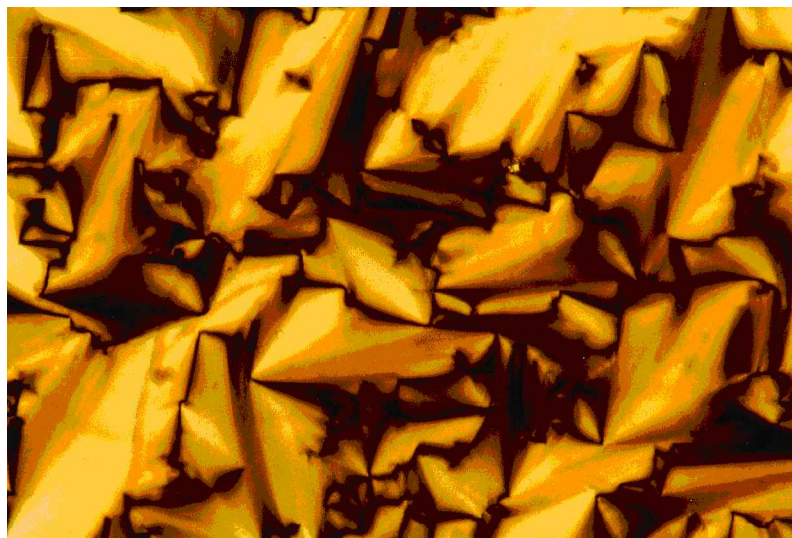
Figure 1. Fan-shaped smectic texture of n -hexadecylammonium pyroglutamate observed on cooling from the isotropic melt ( \times 200 ).
